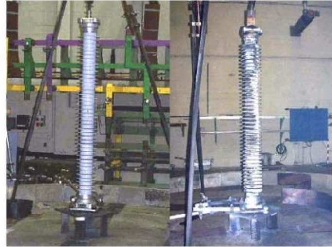
Short circuit behaviour of a porcelain design (left) and polymer tube design surge arrester (right)
