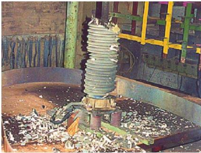
Short circuit behaviour of a porcelain design (left) and polymer tube design surge arrester (right)
